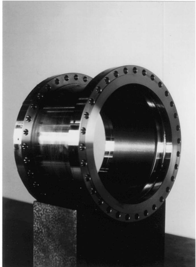
Figure 8.34: A Full size model of the ferrite absorber. The powder of IB-004 ferrite was sintered and bonded to a Cu pipe by HIPping.
