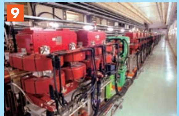
9 Wiggler magnet: This special magnet suppresses beam oscillations by taking advantage of, and strengthening the effect of, the beam's own damping mechanism called "radiative damping."
