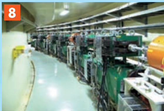
8 Beam transport line: Beams are delivered from the injector to the storage ring by the beam transport line. The delivery line consists of upper and lower lines for delivering positron and electron beams, respectively.
