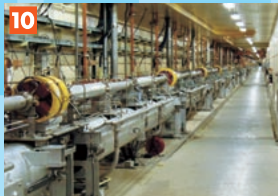
10 Injector: The powerful linear accelerator provides KEKB's double rings with 8 billion electron-Volt electron beams and 3.5 billion electron-Volt positron beams. The injector is a multi-purpose accelerator, also feeding beams to other electron accelerators located at KEK.
